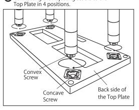
Align the Concave Screws on the back of the Top Plate with the Convex Screws on the Adjusting Blocks, and tighten clockwise until you feel a click.
