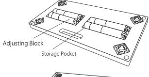
② Put the Stoppers in the Stopper Storage Pockets (refer to method 4 in the instructions for assembly) and tighten the Handles and the Fixing Screws to fix the Plates.
