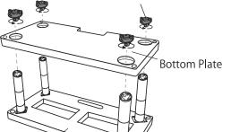
Remove the Adjusting Blocks from the Top Plate (refer to the instructions for assembly methods 3 and 2) and connect the Adjusting Blocks (S), (M) and (L) (4 sets) and store them in the Storage Pockets.
